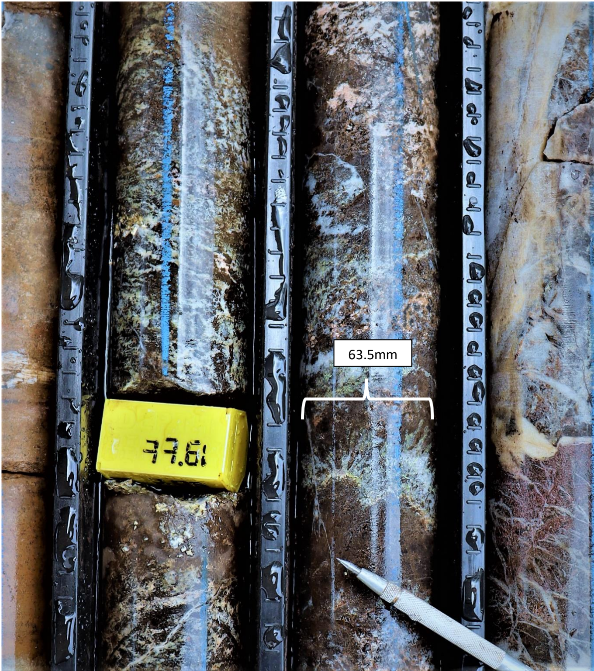
Extensive pale green monazite seen in drill core. The radial pattern above the pen (and below the scale bar) is a large radial cluster of monazite minerals. This drill core specimen has similarities to radial monazite mineralisation in the image below. The blue line is the marker for core cutting and sampling. Yellow marker is 77.61m down hole.
