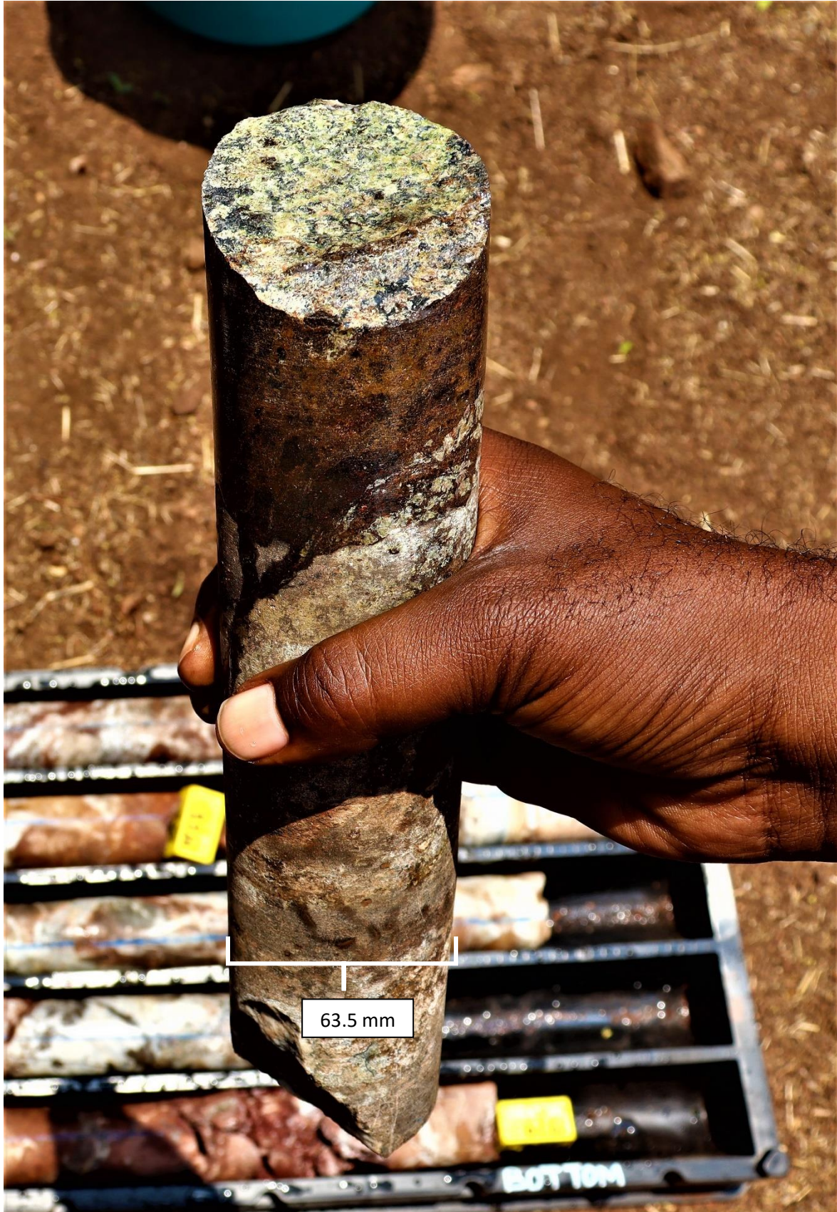
Program geologist with a portion of drill core with pale green monazite mineralisation.
