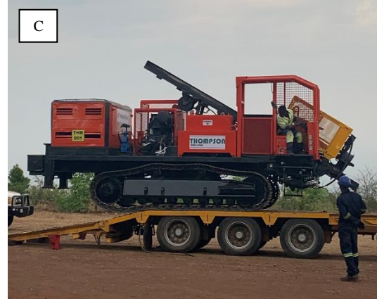
Image C: Second RC rig arrives on site
