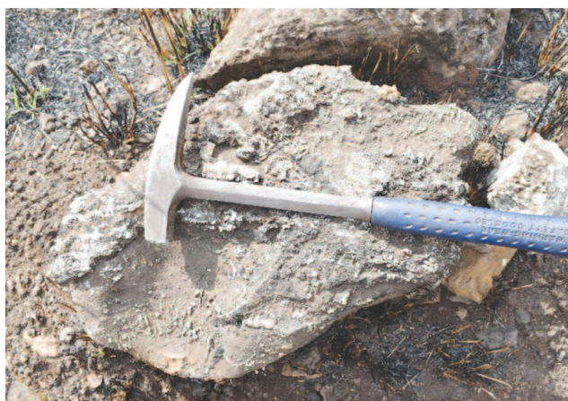
Top left: Lindian Chairman Mr Kabunga with mineralisation near the old plant area at the base of the Kangankunde Hill. Top right: Agglomerate (camera lens cap is 55mm in diameter). Bottom left: large monazite crystals with long handle Estwing hammer as scale (42cm long). Bottom Right: Large radial monazite crystal growth about 12cm in diameter.
