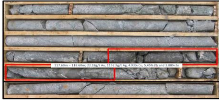
MVS – Drill hole BML-004 with mineralised interval from 117.6 to 118.6 metres. Interval averages 1 metres grading 22.18g/t gold and 1,152.9g/t silver.
