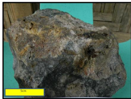
Jasperoidal boulder from Lunar-Magbanua Prospect. Assay grade ranges from 2.68g/t to 8.41g/t gold.
