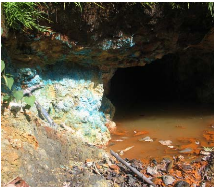
Old copper workings at the Sabang Prospect showing secondary copper exposed at surface.
