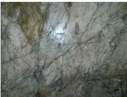
Covellite-bornite vein stockwork and disseminated style mineralisation. Adit 1, north face, Sabang Prospect (1.70% copper, 0.18g/t gold and 5g/t silver).
