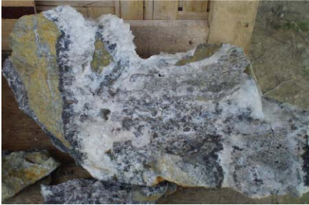
Quartz-gold-silver-galena-sphalerite-chalcopyrite mineralisation, Davaoeno Mine Prospect. The sample is typical of high grade gold mineralisation sampled by Lindian and historically mined in the Davaoeno Shaft.
